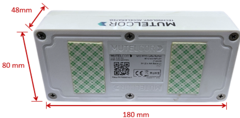
Mounting with 3M Double sided tape
