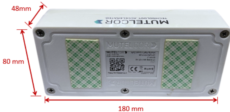
Mounting with 3M Double sided tape
